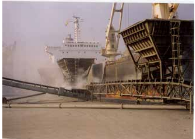
Dust emissions during unloading operations at a terminal on the West Coast of Africa.
