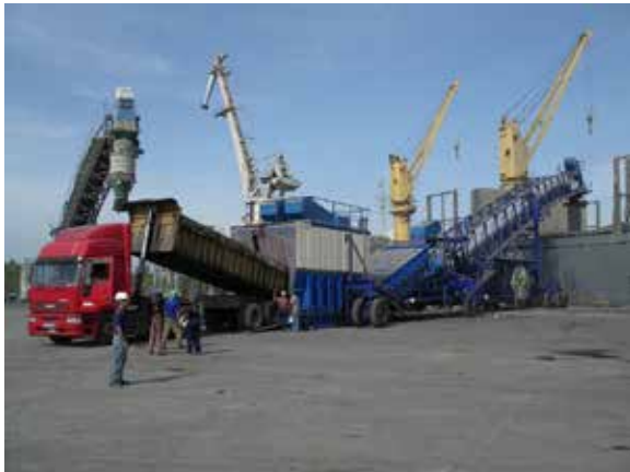
Figure 6. Mobile ship loader (Taim Weser).
