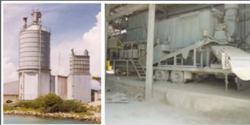
Figure 2: temporary bulk cement import terminal – road-mobile packer (right) and second-hand steel silo (left)
